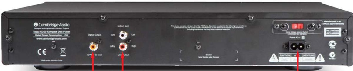
S/P DIF co-axial digital output      RCA line output      AC Power Socket
